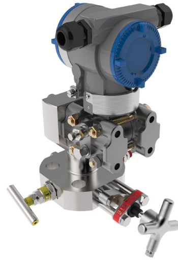
Close-Coupled Double Block and Bleed MONOFLANGE with IEC 61518 TYPE B Outlet connection (not differential) Vertical Mount . Primary OSY isolate, standard needle valve in secondary isolate and vent, with 1/4" NPT plugged vent outlet.
