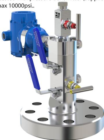
**9.5mm through bore single block and bleed.** Primary ball valve with 1/4" NPT plugged needle vent valve. Rated per flange rating to max 6000psi.
