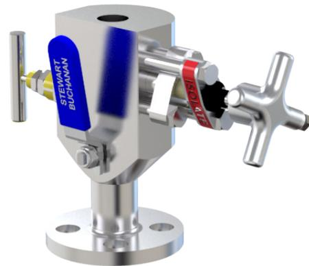
**9.5mm through bore double block and bleed fire safe manifold.** Primary/Secondary and vent ball valves. Rated per flange rating to max 6000psi.
