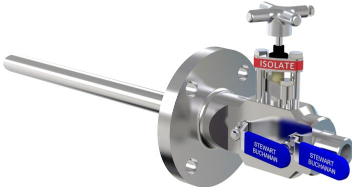
**4.8mm bore with sampling quill.** Primary isolate needle, secondary isolate rising plug, with 1/2" NPT captive bleed plugs and auxiliary ports; assembled and tested with 3 way switching ball valve for flushing and sampling. Rated per flange rating to max 10000psi.
