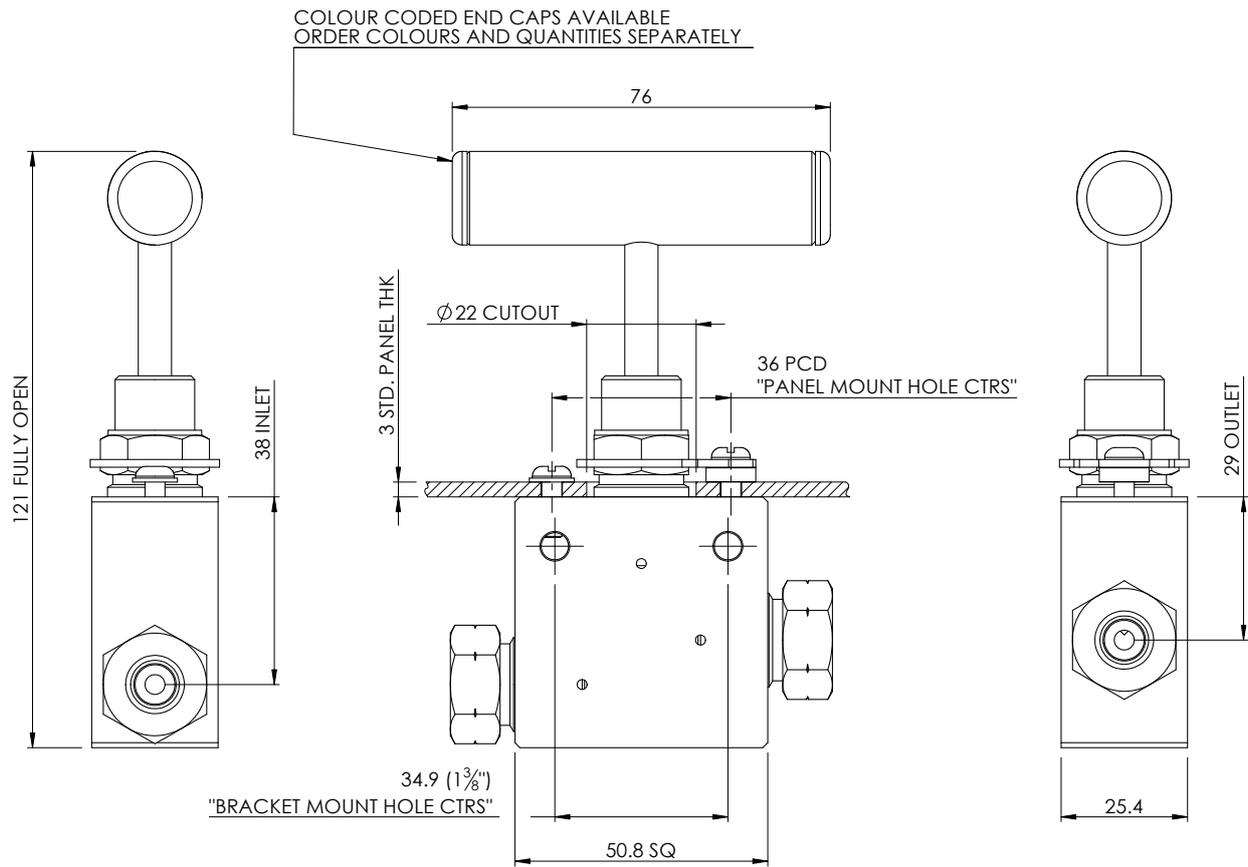
1/4" and 3/8" MP and HP Valve Geometry
