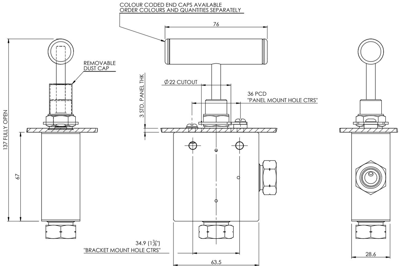
Right Angle 9/16" Medium Pressure Valve Geometry
