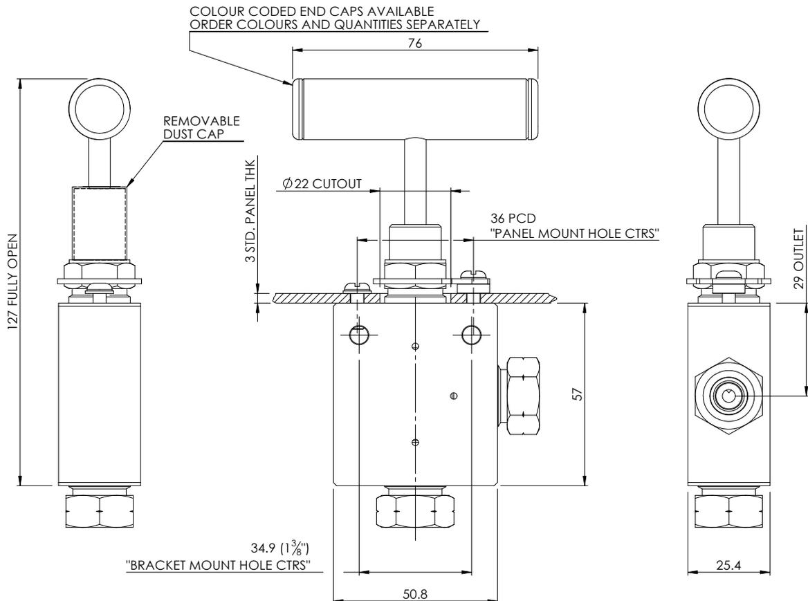
Right Angle 3/8" MP & HP Valve Geometry
