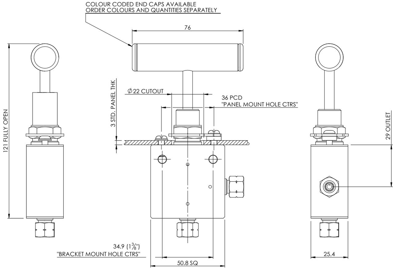
Right Angle 1/4" MP & HP Valve Geometry
