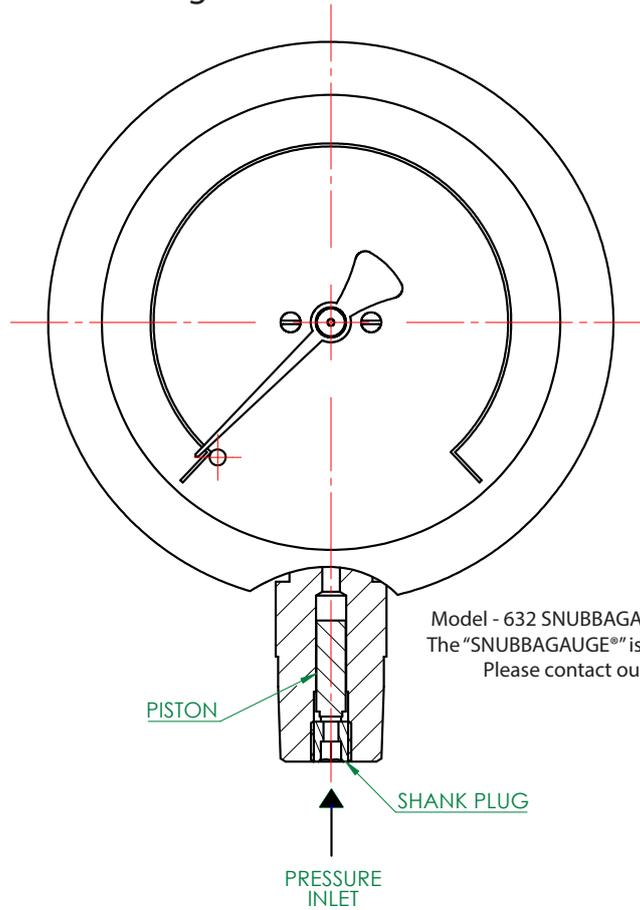
Model - 632 SNUBBAGAUGE® (100mm,4" Direct Mounted (Standard))
