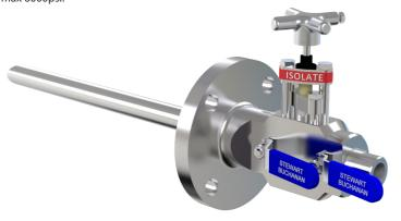
4.8mm bore with sampling quill. Primary isolate needle, secondary isolate rising plug, with 1/2" NPT captive bleed plugs and auxiliary ports; assembled and tested with 3 way switching ball valve for flushing and sampling. Rated per flange rating
