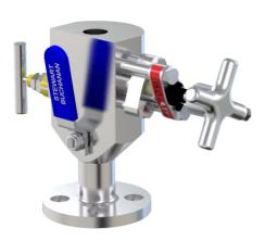
9.5mm through bore double block and bleed fire safe manifold. Primary/Secondary and vent ball valves. Rated per flange rating to max 6000psi.
