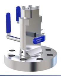
**9.6mm bore double block and bleed manifold.** Primary isolate needle, secondary isolate rising plug valve, with 1/2" NPT captive bleed plugs and auxiliary ports. Rated per flange rating to max 6000psi.
