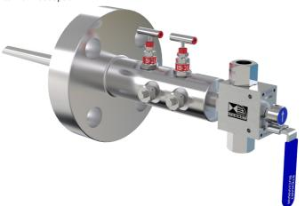
9.5mm through bore with API Flange sampling rising plug valve. Primary/Secondary ball valves and 1/2" NPT plugged needle vent valve, additional 1/2" NPT auxiliary port; assembled and tested with pressure transmitter (supplied by others) Rated
