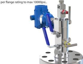
9.5mm through bore single block and bleed. Primary ball valve with 1/4" NPT plugged needle vent valve. Rated per flange rating to max 6000psi.
