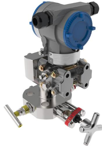
*Close-Coupled Double Block and Bleed MONOFLANGE with IEC 61518 TYPE B Outlet connection (not differential) **Vertical Mount**. Primary OSY isolate, standard needle valve in secondary isolate and vent, with 1/4" NPT plugged vent outlet.*
