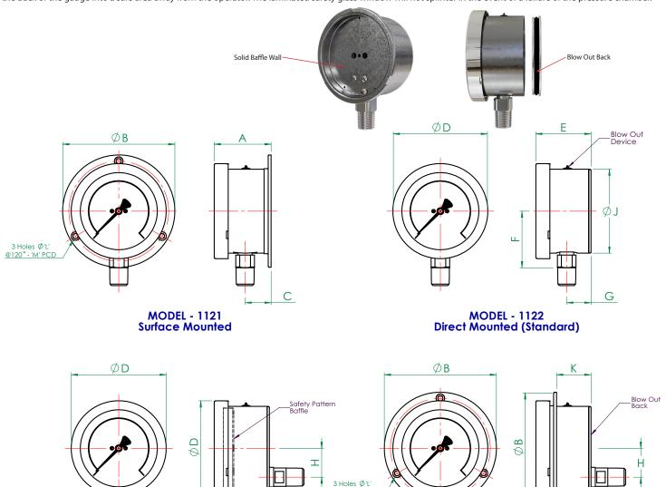
$Surface\ mounted\ gauges\ should\ be\ fitted\ with\ distance\ pieces\ of\ not\ less\ that\ 3/4'' (20mm)\ long\ to\ allow\ them\ to\ be\ mounted\ away\ from\ wall\ or\ panel.$
