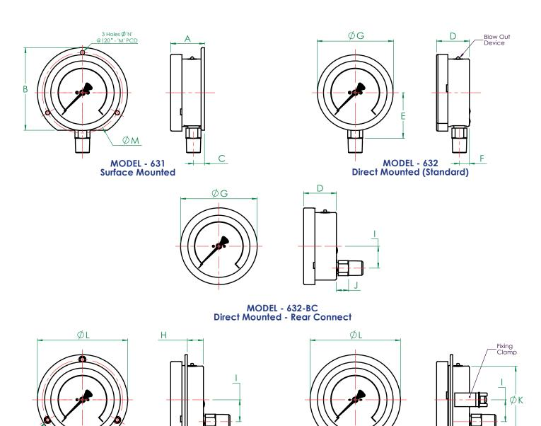
3 Holes Ø'O' csk @120°- 'M' PCD MODEL - 633 Flush Mounted - Screw Fixing
