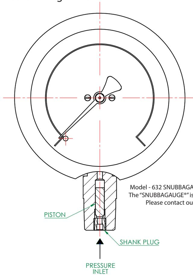
Model - 632 SNUBBGAUGE® (100mm,4" Direct Mounted (Standard))
